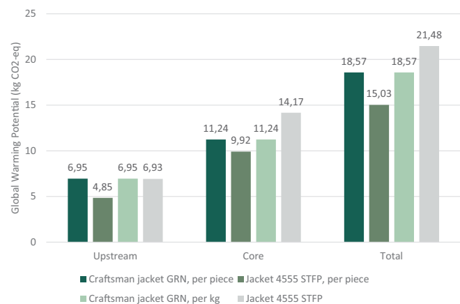
Figure 3. The Global Warming Potential of Craftsman jacket GRN and Jacket 4555 STFP. Figures per jacket and per kg of jacket.
